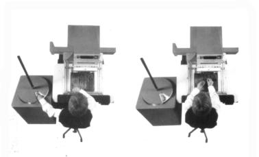
The bin opening is conveniently located next to the board fixture. The operator picks up a quantity of parts with one hand and inserts with the other. (Light curtain removed for clarity).
