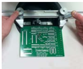
The Operator clamps the next PC board on the Workfixture
