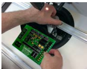
The Operator removes the completed PC board from the Workfixture
