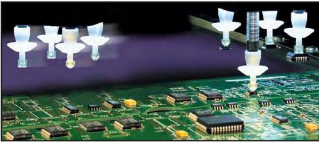
Both four spindle heads can place all components from 0201 to fine pitch QFP's.
