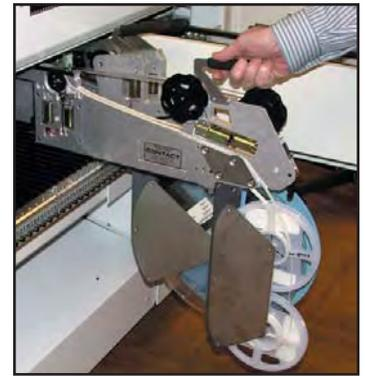
Smart tape feeders eliminate kitting errors. The compact design enables maximum density, and are available for all tapes from 8mm to 56mm.
