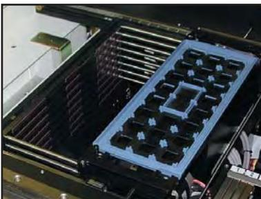
**Auto-centering conveyor** positions the board at the center of the placement area so the picking head is unimpeded by the placing head, thus assuring non-stop placements.
