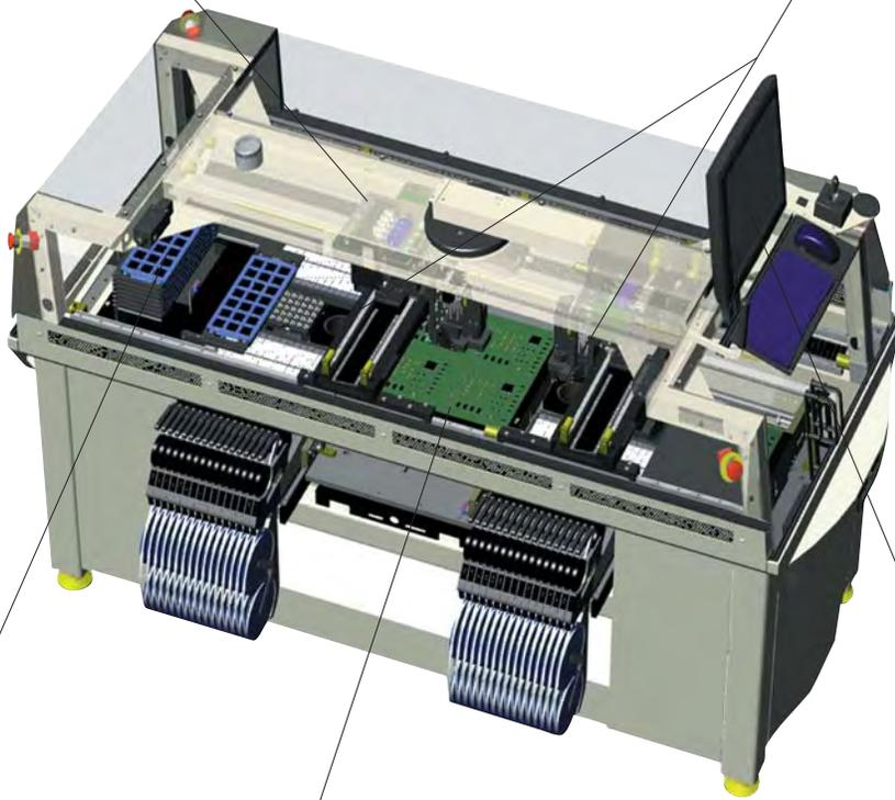
The optional **eight tray magazine** mounts within the machine and feeds trays between the feeder banks without loss of feeder capacity.
