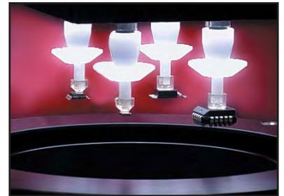
Vision cameras are centrally positioned for **"fly by centering"**. Backlighting provides high contrast silhouette component image for robust vision processing.
