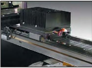
Advanced gantry design uses linear motors and encoders in both the X and Y axes --- Unlike ball screw systems, **linear motors** have zero backlash and require no maintenance....ever.
