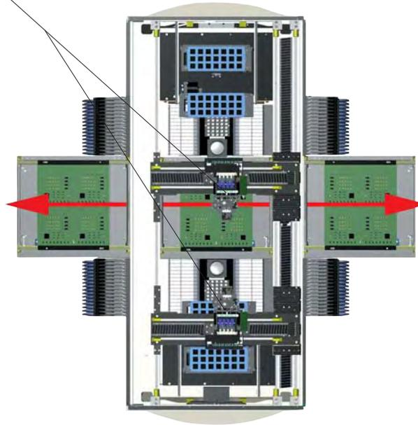
The air track stick feeders provide reliable feeding (unlike vibratory feeders), easy track changeover, and easy on-line replenishment.
