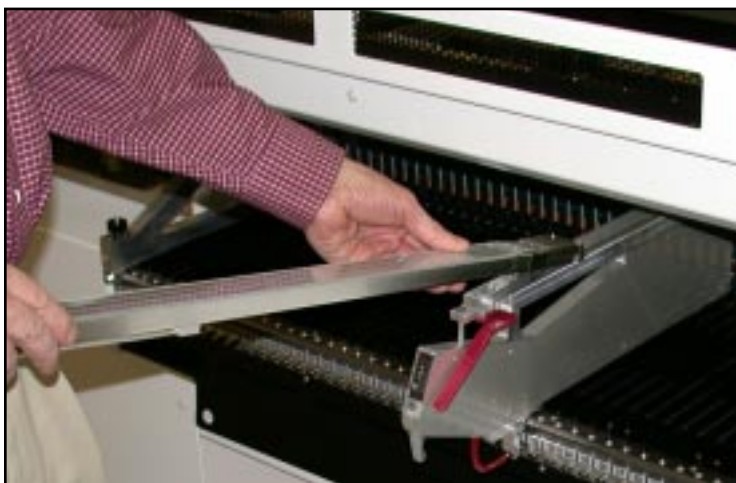
Track are easily removed and replaced while on the machine
